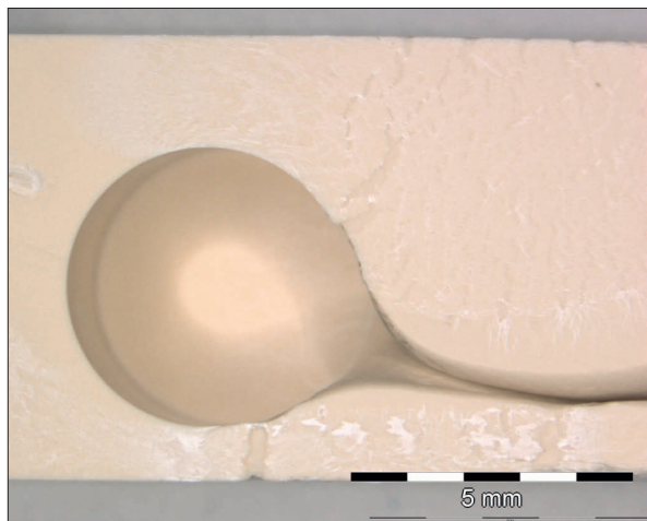
Fig. 2 Real mold filling experiment based on the injection parameters of the simulation (Fig. 1)
