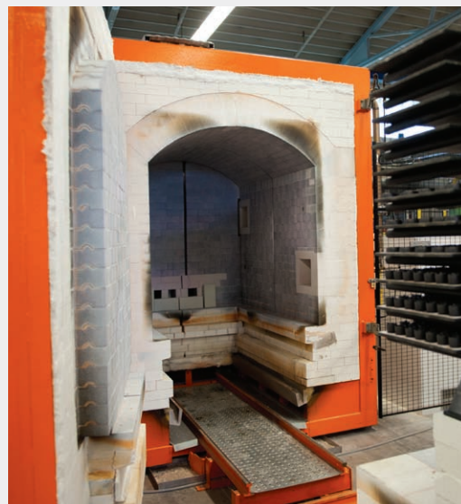
De-binding and sintering in the ceramic furnace
