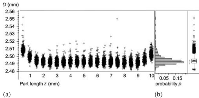
Fig. 4. Distribution of measured outer diameters (11510 values) of 160 sintered parts over (a) part length and (b) as a histogram with outlier box plot.
