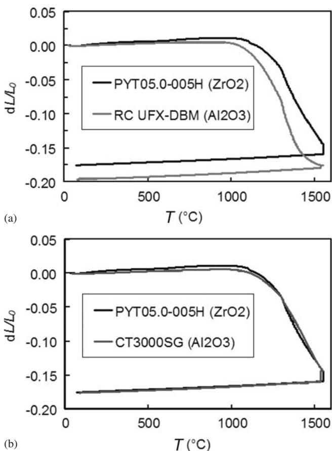
Fig. 6. Relative length changes of selected  $\text{ZrO}_2/\text{Al}_2\text{O}_3$  powders during sintering. (a) combination promising for mobile bonds, (b) possible combination for an immobile bond.
