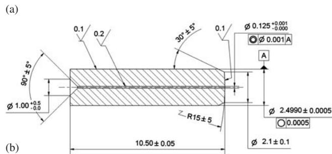
Fig. 3. (a) Stages of the CIM process: green compact (1), brown part (2) and sintered part (3) of single-mode ferrule, (b) product specification for single-mode ferrule (dimensions in mm).
