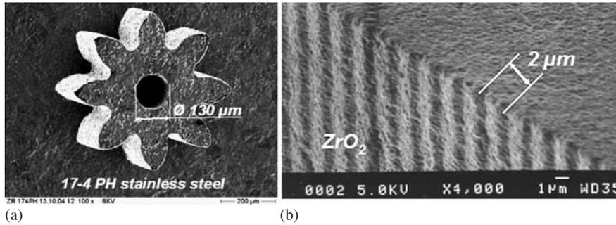
Fig. 1. Sintered LIGA test structures made by Powder Injection Molding. (a) Gear wheel in stainless steel 17-4PH, (b) Spectrometer test structure with a step height of approx. 0.8 μm in zirconium oxide.
