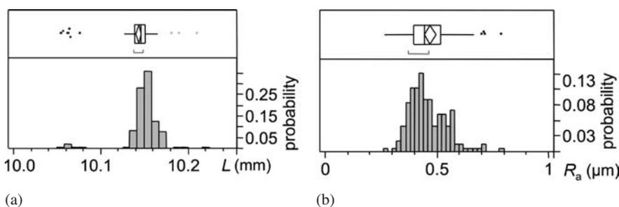
Fig. 5. (a) Distribution of measured lengths of 160 sintered parts, (b) distribution of measured average roughness  $R_a$  of 160 sintered parts.
