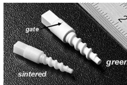
Fig. 2. (a) Scheme of the new molding tool operating with screw-out demolding procedure, (b) Samples of screws as in the sintered state and as green bodies just after demolding by unscrewing and ejection.
