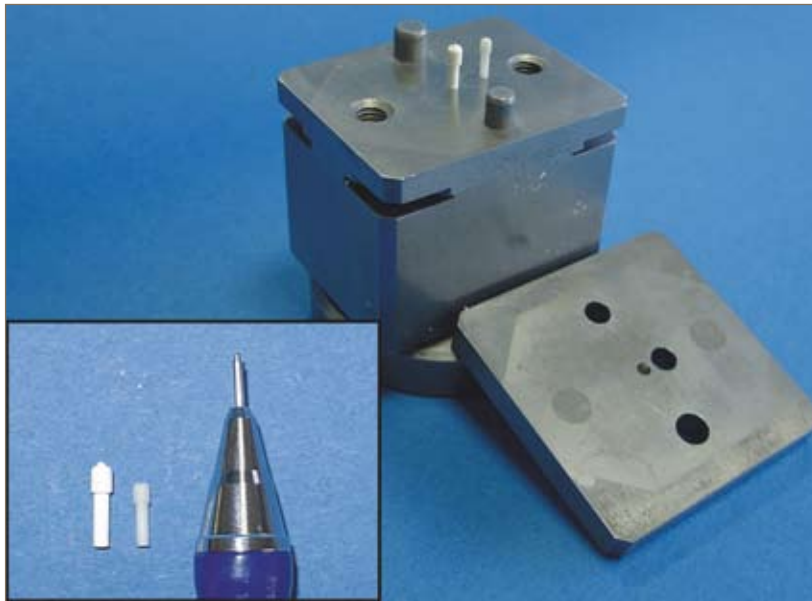
Fig. 3 Nozzle body for cooling systems of power stations with hot moulding tool (Courtesy MicroCeram GmbH)
