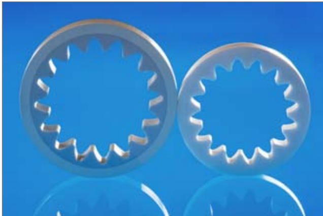
Fig. 5 Ceramic gear wheel in the green and sintered state made by two-component CIM combining alumina and zirconia toughened alumina (Courtesy Fraunhofer IKTS, designed by Robert Bosch GmbH)
